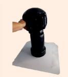
3. Subsequently, we will install the ventilation head on the vent and trouble-free its operation. The head must be mounted in a vertical position, otherwise there is a risk of uneven wear of the bearing and the turbine may not perform its function properly..
