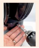
4. Securing the head against blowing away is done by means of three self-tapping screws, which are inserted into pre-prepared holes.
